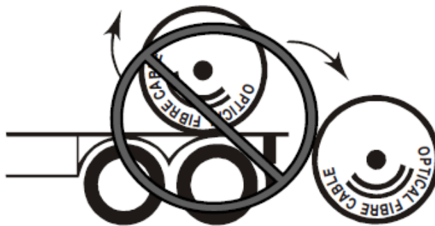
Figure 4-13 Loading/Unloading of Cable Drum
