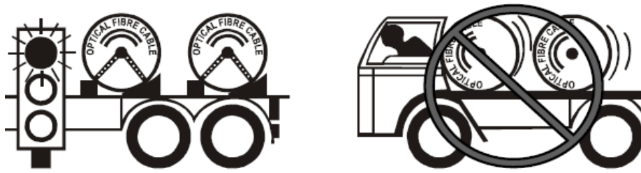
Figure 4-10 Cable Drum Loading
